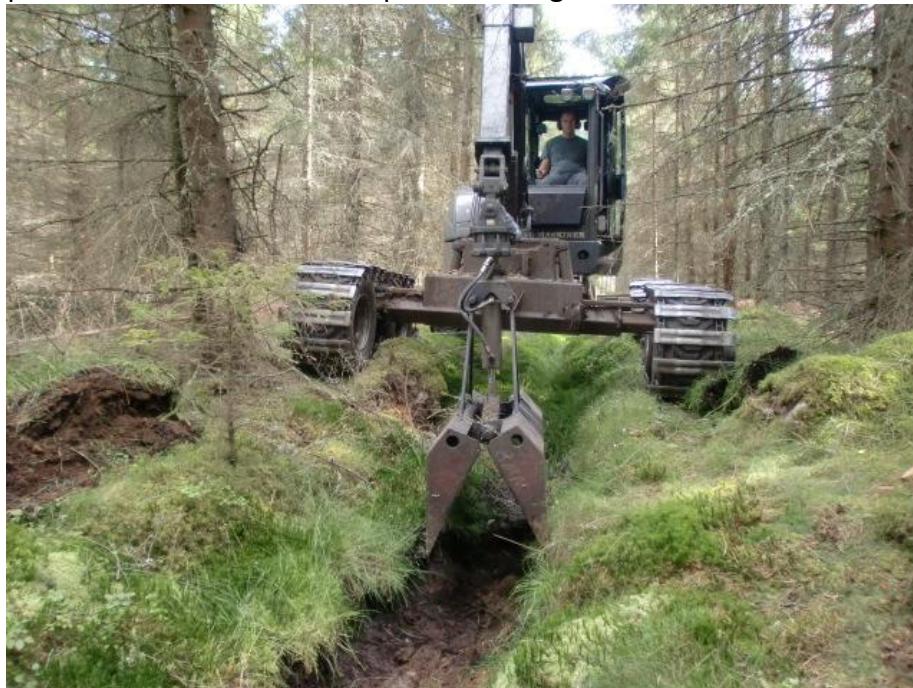
Figure 1. A new machine innovation called “Varanen” carrying out ditch network maintenance in Sweden. Photo by Anja Lomander.
